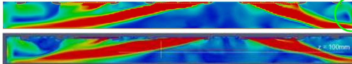
Problem with boundary condition that needs to be rectified and which explains the low horizontal gradient in T
